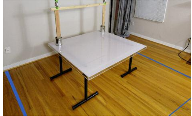
The photo studio requires about 8' x 10' clear space, as shown by blue lines on floor. My table has 44" x 48" top resting (not connected) on adjustable height IKEA legs. Two 2' Stick-In-Cans are on table.
