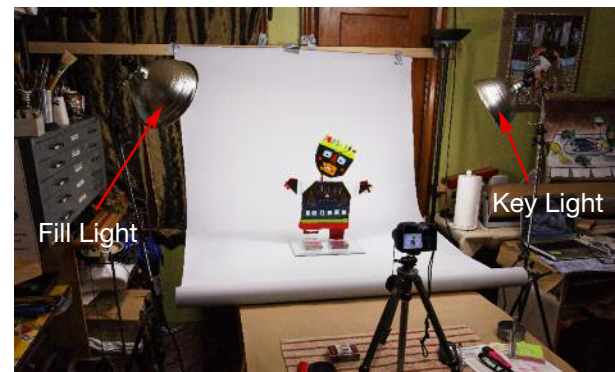
You don't need a fancy setup. This real artist's studio uses two lights and a roll of seamless grey paper. A Key Light and Fill Light are placed right and left of the art object to reflect off the background. Spill light also falls on the front of the object.
