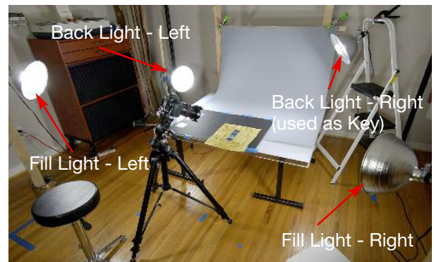
Side Lighting Setup: Lights are positioned around the object at various distances to create interesting shadows. One or more side lights can be used (or added to overhead light).
